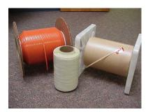
Winders, unwinders, spoolers and tension controllers can be found in many applications in the **converting** industry. For narrow or wide **web handling**, controls must handle large changes in roll diameter and inertia. For **wire spooling** or **level winding**, an additional traverse axis is required to move product across the spool.
